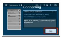
2 Wifi connection, turn on the "Easy connection Application", select wifi connection icon, then creat a wifi hotspot on headunit, after that connect mobile to the hotspot, then screen mirror will appear.
